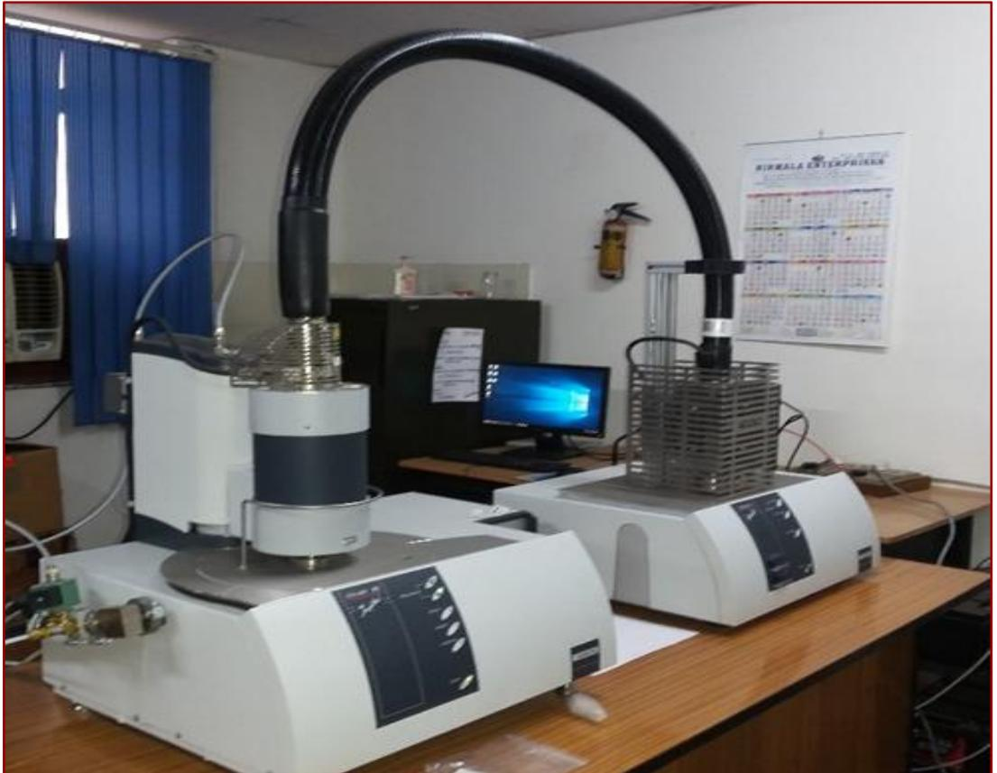
Thermo-Gravimetric Analyzer and Quadrupole Mass Spectrometer will be used in studying and characterizing the thermal properties such as mass change, thermal decomposition, evolved gas analysis for a wide variety of samples from minerals to synthesized metal/metal oxide/polymeric/Organic and inorganic compounds.
