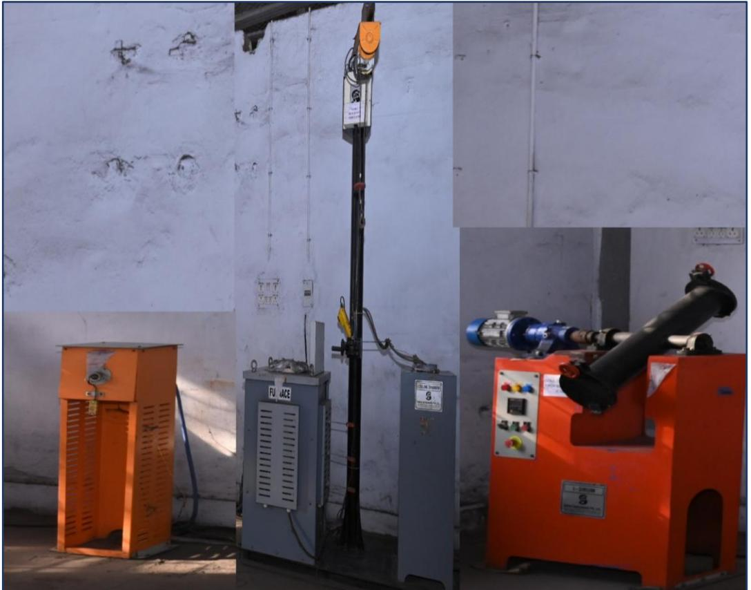
The equipment measures (i) Coke Reactivity Index (CRI) and (ii) Coke Strength after Reaction (CSR), indicative of the performance of coke in the Blast furnace. 200 g of sample is heated with  $\text{CO}_2$  at  $1100^\circ\text{C}$  in a retort, followed by tumbling. The percentage of mass loss gives CRI, and the percentage of + 10 mm particles retained by tumbling gives CSR as per ASTM protocol. The data is useful in determining coal quality for blast furnace applications.
