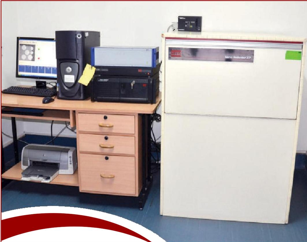
This XP naniondenter works in continuous stiffness measurement (CSM) and control load mode. Berkovich indenter is mainly used for the determination of mechanical properties and elastic-plastic behaviour of materials. It has nano vision and DCM attachment, also for related studies. The Load range in XP and DCM mode is given below
