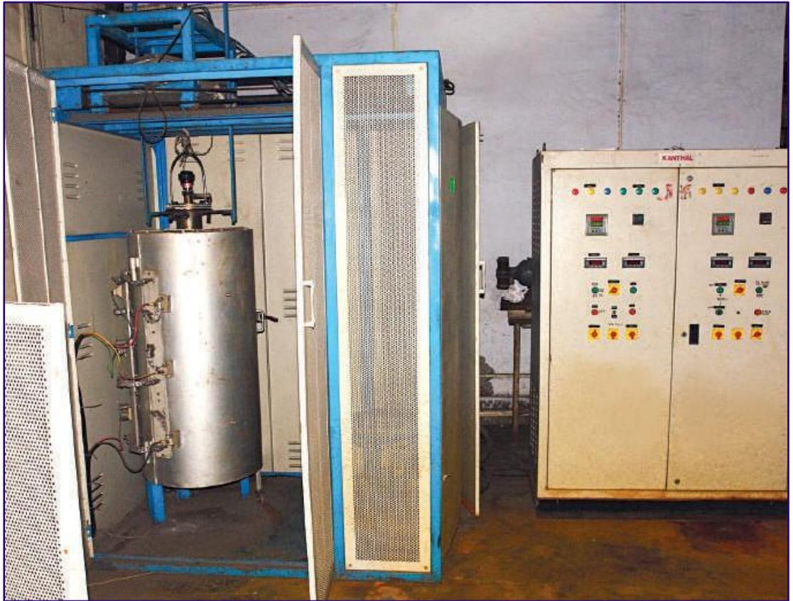
Quality and suitability of using iron ore/agglomerates as iron burden can be estimated prior to its charging in iron making industries. The tests simulate the actual operating conditions.
