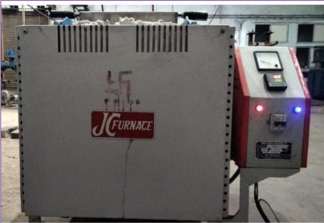
The Aluminum (Al) and Aluminum-Alloys Melting Furnace of 10 Kg capacity is a specialized laboratory apparatus designed for controlled melting and casting of aluminum and its alloys in experimental research. This furnace provides precise temperature regulation, uniform heat distribution, and a stable melting environment, ensuring reproducible results for metallurgical studies.
