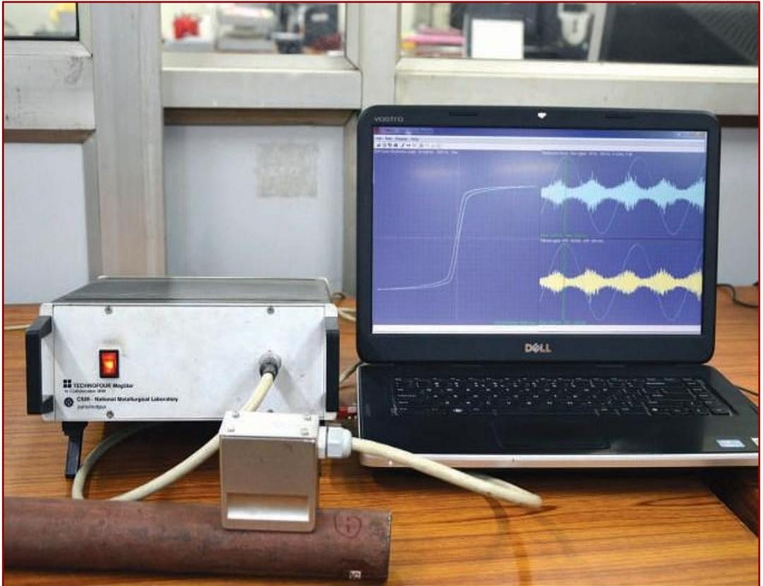
MagStar is a Magnetic NDE device developed jointly by M/s Technofour, Pune, and CSIR-National Metallurgical Laboratory, Jamshedpur. It measures Magnetic Hysteresis Loop (MHL) and Magnetic Barkhausen Emissions (MBE) using a single magnetizing probe. It has also the option for measuring MHL and MBE separately. The device is portable, light weight and has no-line measurement facility.
