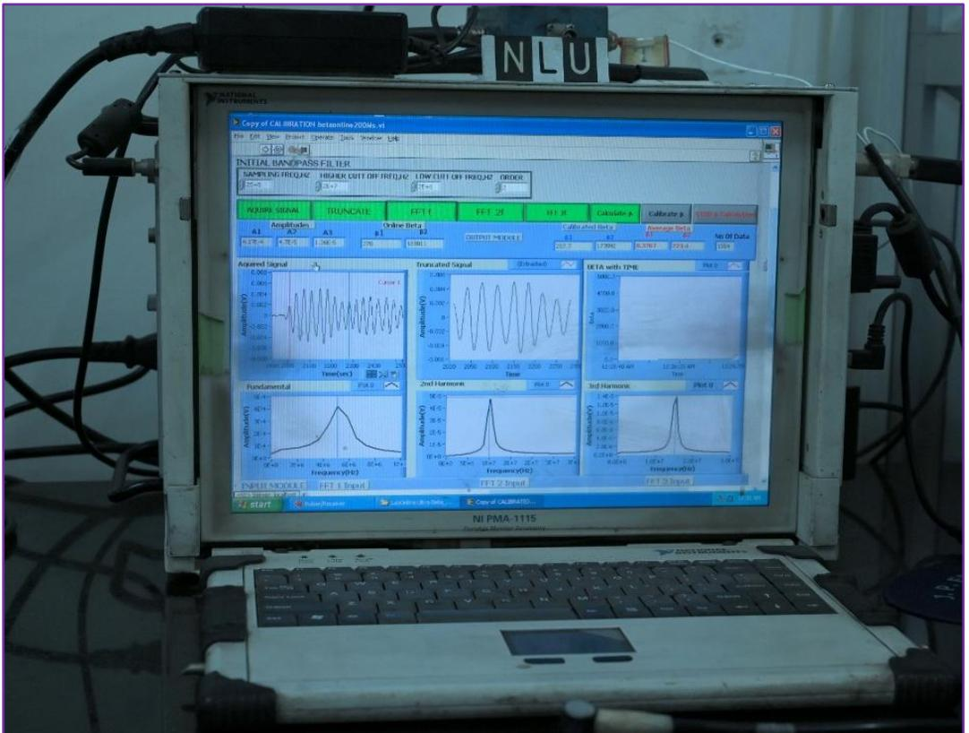
Portable nonlinear ultrasonic device is a single unit solution for concrete to metals. It can be used as conventional ultrasonic system as well as a high power pulser for EMAT, guided wave ultrasonic and nonlinear ultrasonic. Software Cal $\beta$ , has been developed in-house for online NLU parameter determination along with calibration, data saving and report generation modules.
