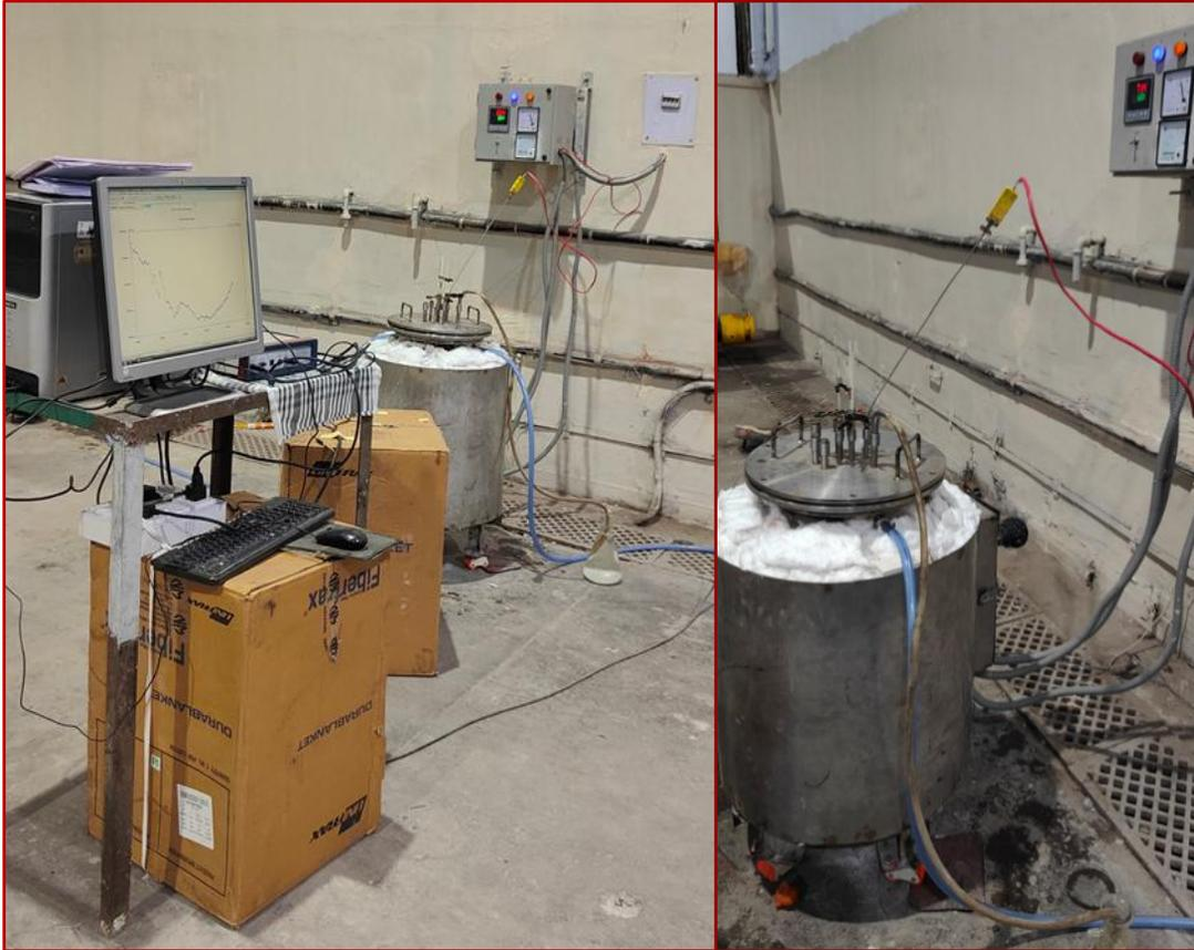
Can be used to examine the corrosion behaviour of the various metal/alloys and coatings in high temperature corrosive environment (especially in molten salt atmosphere).
