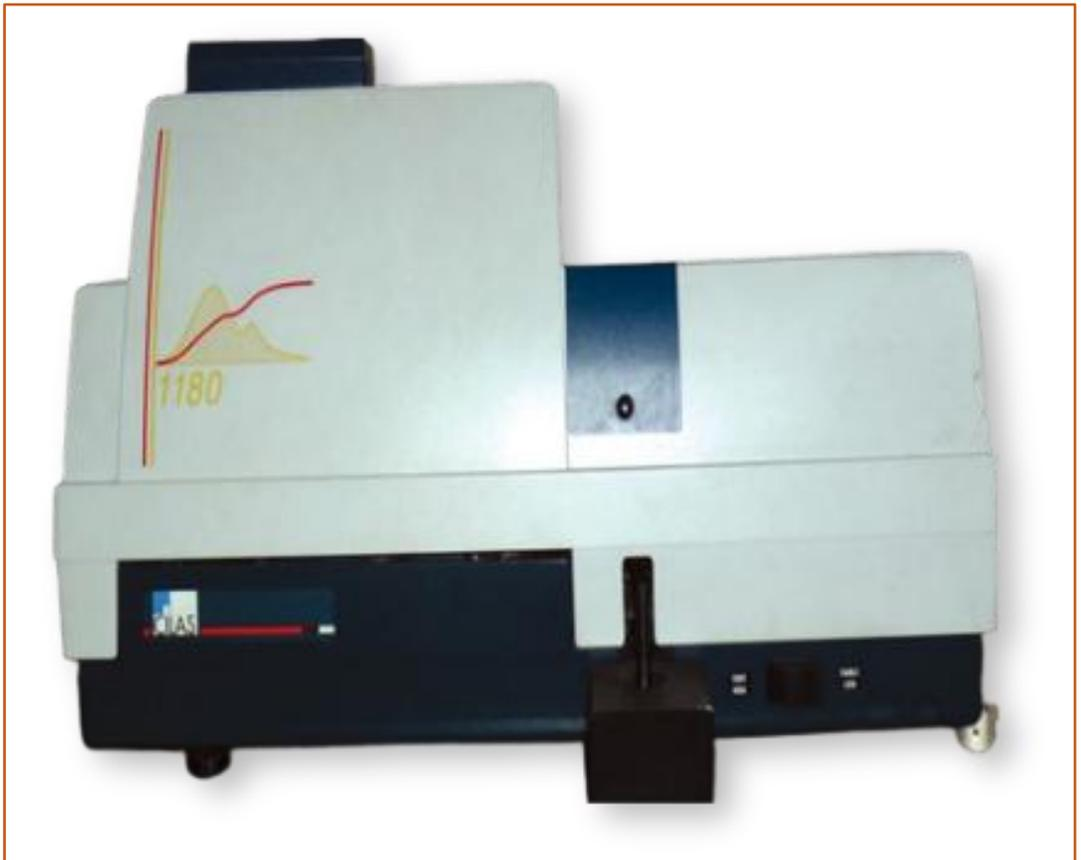
The Laser Particle size analyzer is used to measure the particle size distribution of a sample. It utilizes Helium-Neon laser beam diffraction for the measurement and also considers that the particles are spherical in nature. The analysis involves both dry and wet modes of operation, depending upon the nature and size of the particles. This instrument measures particle size ranging from 0.04 to 2500  $\mu\text{m}$ .
