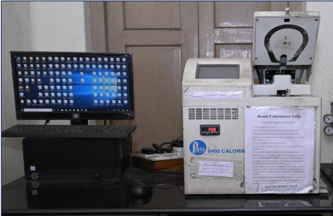
A bomb calorimeter is used to determine the calorific value of fuels. A known amount of the fuels (coal, petroleum products) is burnt inside a stainless-steel bomb in a water bucket containing a known volume of water in excess oxygen. The heat produced by the combustion raises the temperature of the water, which is used to calculate the calorific value of the fuel.
