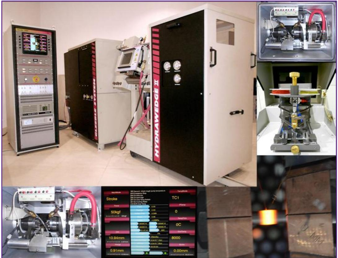
Gleeble 3800™ is an advanced experimental system designed for process simulation, material testing and analyzing the thermal behavior of material under different process condition. It can simulate wide range of processes like welding, casting, forming (Hot rolling and extrusion), Heat treatment (Strip Annealing) etc.
