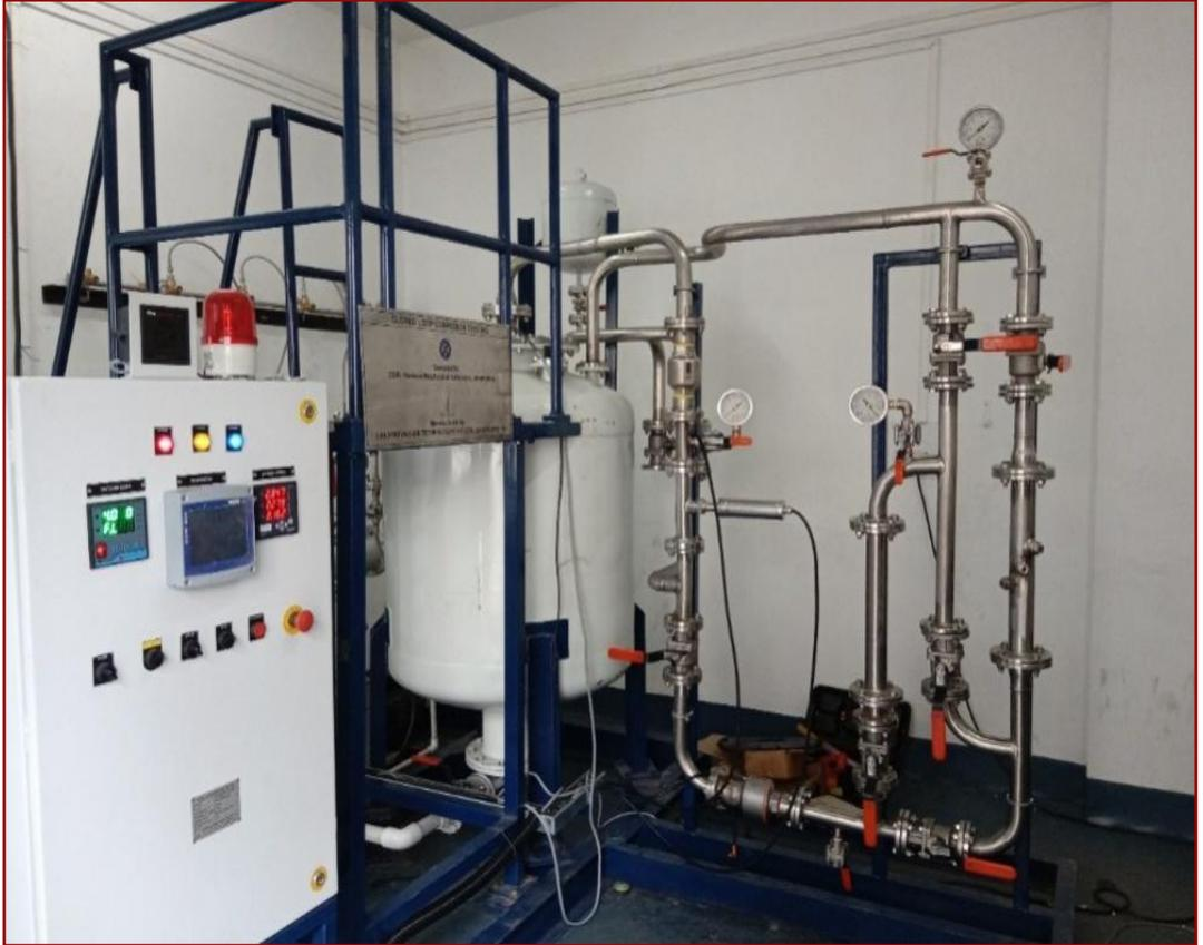
It can be used to simulate the fluid flow and to study the corrosion rate of metals/alloys in the presence of controlled oxygen dissolved in the fluid. The corrosion test rig can be operated/controlled through computer using dedicated software and test data is recorded at set intervals.
