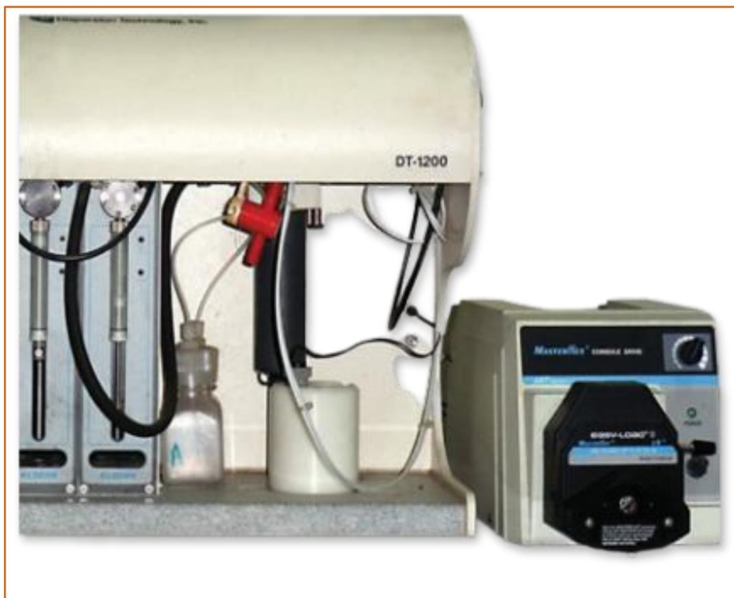
The zeta sizer is a combined acoustic and electroacoustic spectrometer for characterization of particle size and zeta potential of dispersions and emulsions. Zeta potential is determined by measuring colloid vibration current that results from displacement of electrical double - layer of charged particles under influence of ultrasound. The pH range variation is from 0.5 to 13 and particle size measurement ranges from 0.005  $\mu\text{m}$  to 1000  $\mu\text{m}$ .
