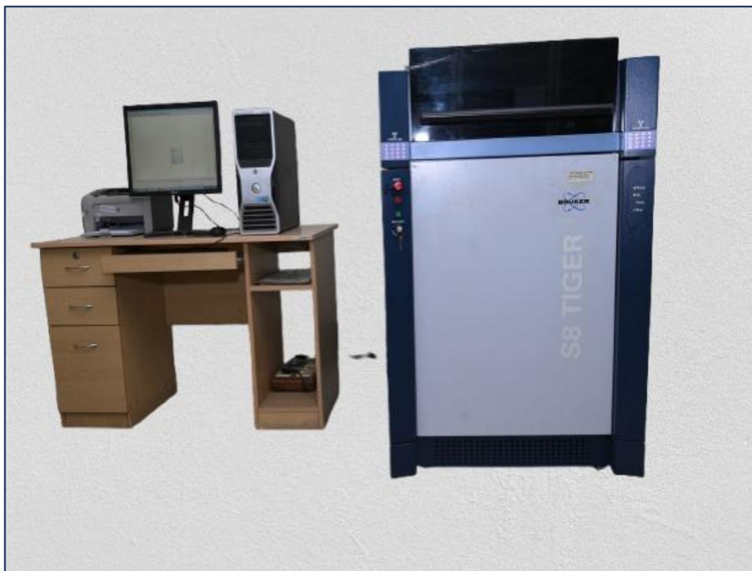
Bruker S8 Tiger is a Fully Automated Sequential WD-XRF for high speed and high precision Qualitative and Quantitative analysis of elements ranging from Beryllium to Uranium, which is used for the analysis of minor & major elements in geological, environmental, metal and alloy samples.
