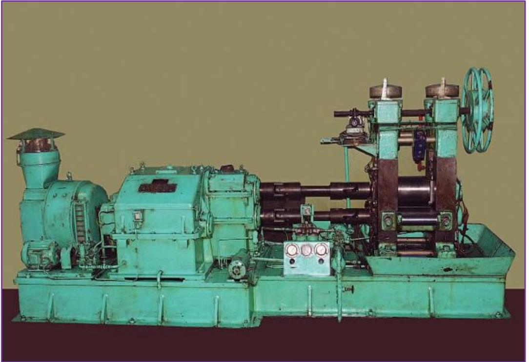
Two high rolling mill: A two high rolling mill for hot and cold rolling for ferrous and non-ferrous metals was built by Hydro-press Inc. The mill stand shown has a pair of 6in. diameter x 10 in. face rolls made of special harden forged steel to with stand hot or cold rolling. Maxim roll gap is 50 mm.
