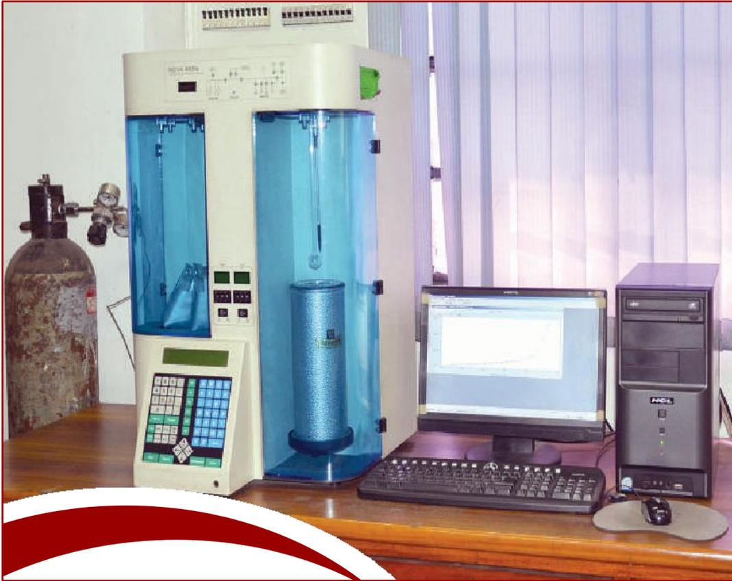
Brunauer-Emmett-Teller (BET) surface area and pore size analysis based on the principle of N<sub>2</sub> adsorption-desorption method at liquid nitrogen temperature. Present equipment offers determination of complete BET analysis includes BET surface area, mesopore size distribution, pore volume and average pore diameter.
