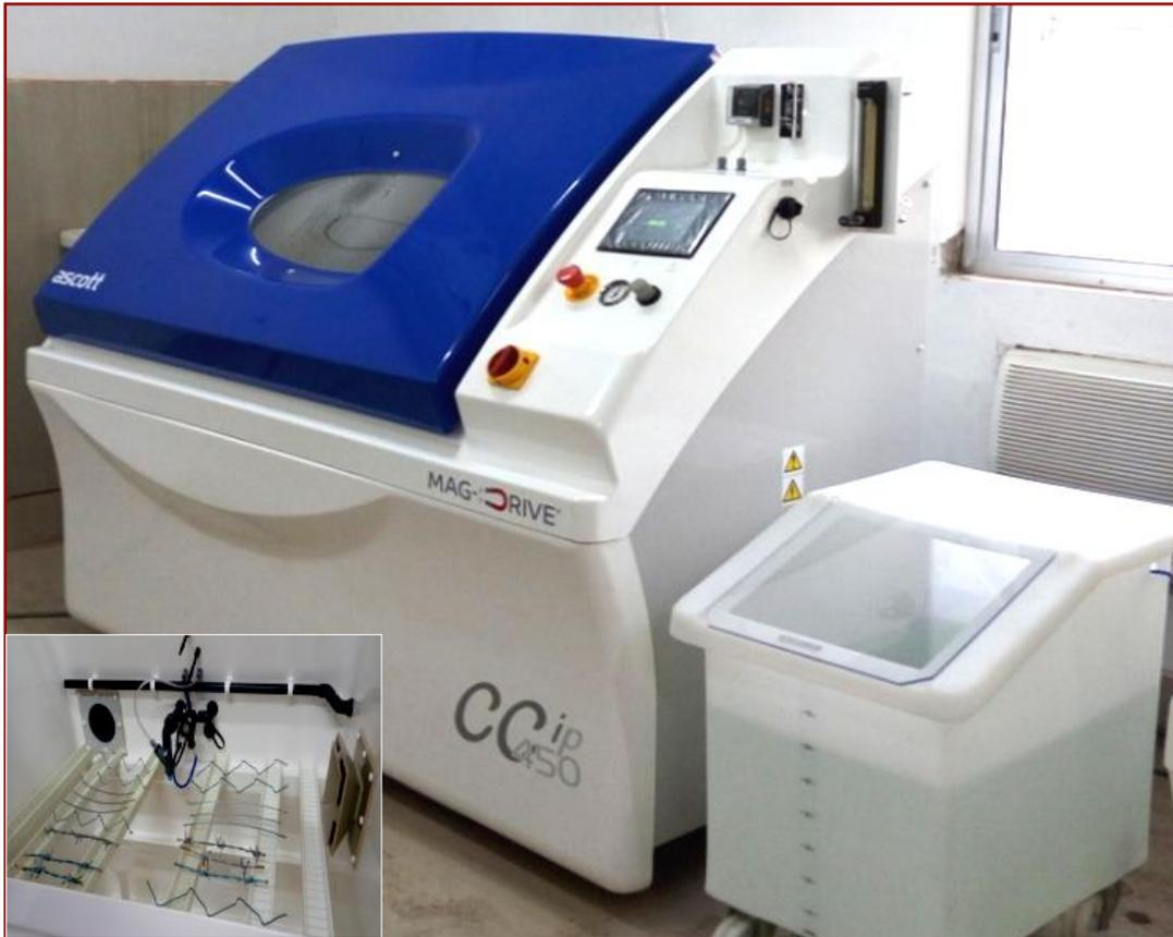
To perform corrosion studies on metals/alloys/nonmetallic materials by means of recreating/accelerating a variety of corrosive climates within the convenience of an enclosed test facility. Facilitates to create 4 distinct climates as follows:
