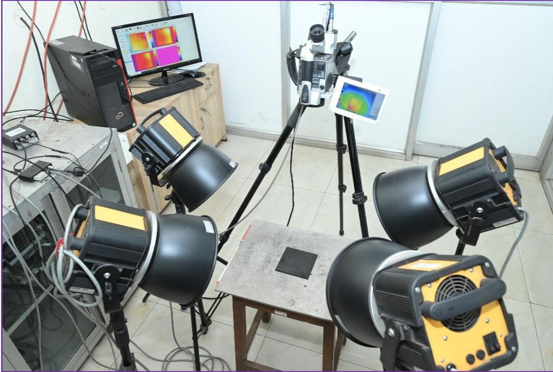
The computer-controlled thermography system is used to detect the inhomogeneities in the sample. Typical field of applications of this system are Material inspections, Quality Control & Process monitoring, Predictive maintenance, Gas Leak detection, thermographic inspection of electrical and mechanical systems and aggregates, Detection of layer structures, delamination and inserts within plastics, composites, etc.
