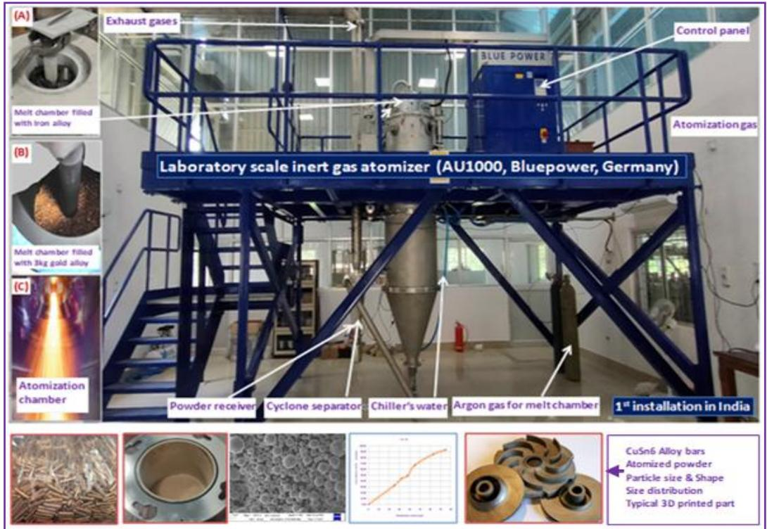
CSIR-NML, has taken a lead role to realize “Self-reliant India”, and setup a state-of-the-art “Laboratory scale Inert Gas Atomizer (IGA)” facility in India. This unique facility is aimed at leveraging:
