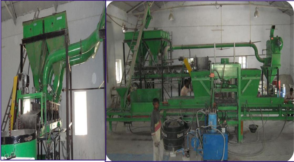
Fully automatic Pilot Plant for block, brick, briquette making
