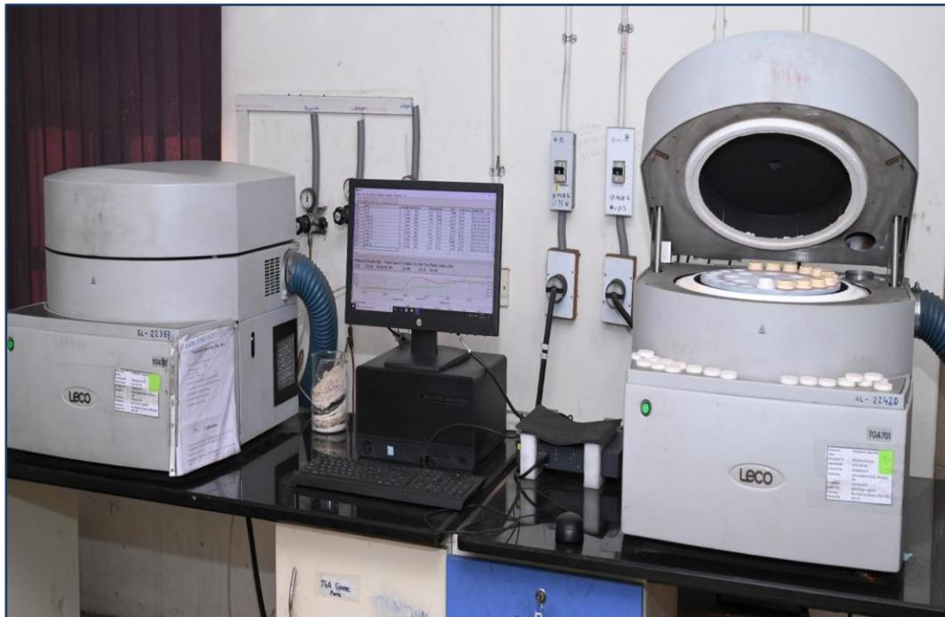
Proximate analyzer is used for proximate analysis of coal. The instrument determines the moisture, Ash, Volatile Matter, and loss on ignition content of coal by measuring the weight loss at different temperatures in controlled environment. 19 samples can be analyzed simultaneously in selectable Nitrogen, Oxygen or Air atmosphere.
