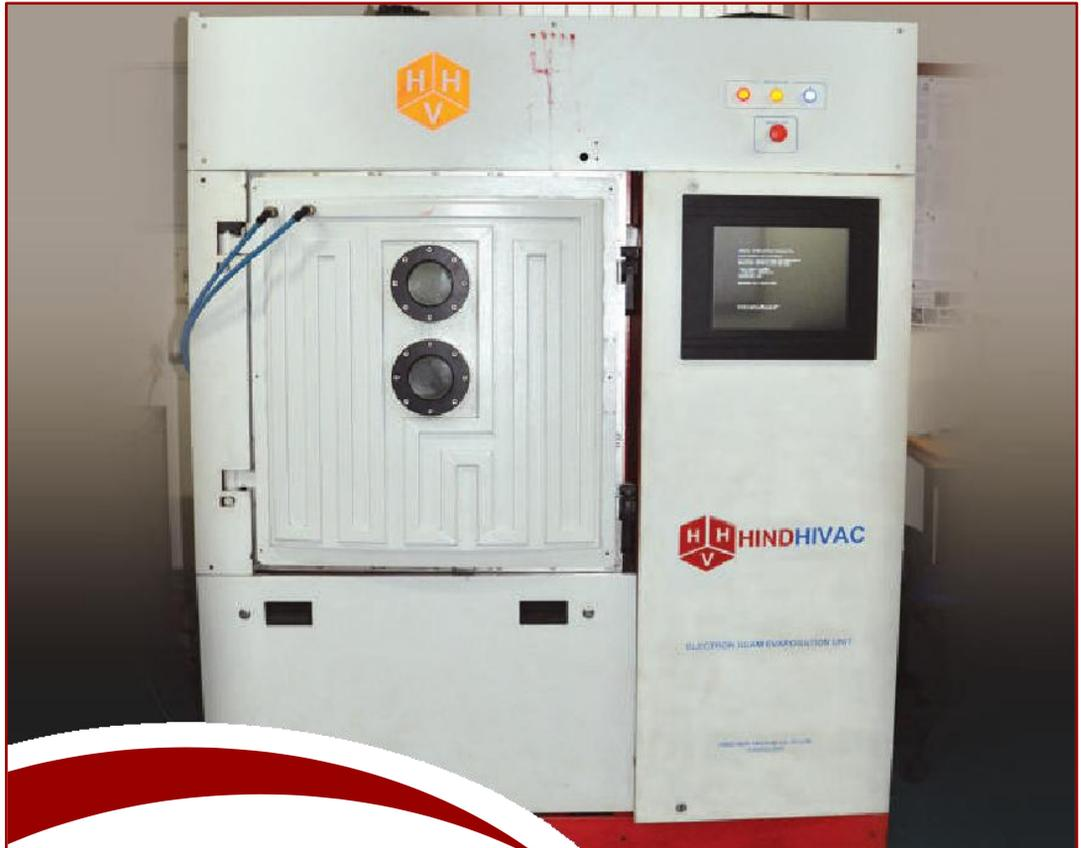
Electron beam evaporation is used for coating single layer and multilayers of metals, alloys, and ceramics. It is an atomic deposition PVD process, done by Thermal evaporation, where the coating material is melted with the help of an electron beam gun. The unit has the capability of  $1 \times 10^{-7}$  mbar. It has 2 electron guns having 4 crucibles in each. The substrate (on which coating is required) also has a heating facility up to 700°C.
