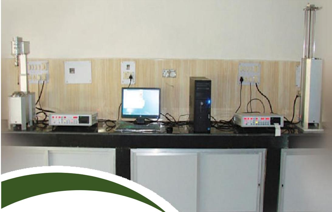
The equipment measures the plastic and dilatation properties of coal on heating as per ASTM protocol. It also measures softening temperature, resolidification temperature, and temperature of maximum fluidity. The data is useful in engineering applications of coal in carbonization, gasification, liquefaction, and combustion.
