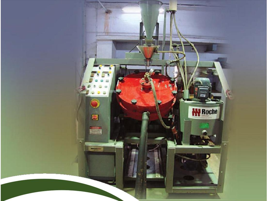
Kelsey Centrifugal Jig is an enhanced gravity separator which allows separation of mineral particles in the fine size ranges. The Kelsey Jig is based on the principles of conventional mineral jig but operates at g-force 100 times that of gravity. This results in improved separation efficiency particularly in fine sizes. The feed particle size to be treated by Kelsey Jig should be < 500 micron.
