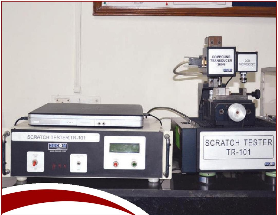
The indenter drags on the surface of the sample with different loads. By using the traction force and normal load, one can find the coefficient of friction. The Rockwell indenter is used for the purpose
