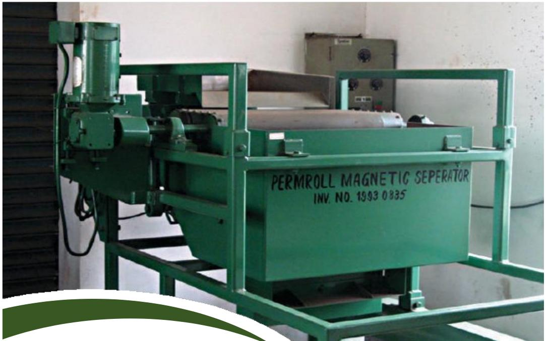
Each ore mineral has definite and different magnetic susceptibilities which is exploited through magnetic separation to separate either valuable magnetic minerals from non magnetic gangue minerals or magnetic impurities from valuable non-magnetic minerals.
