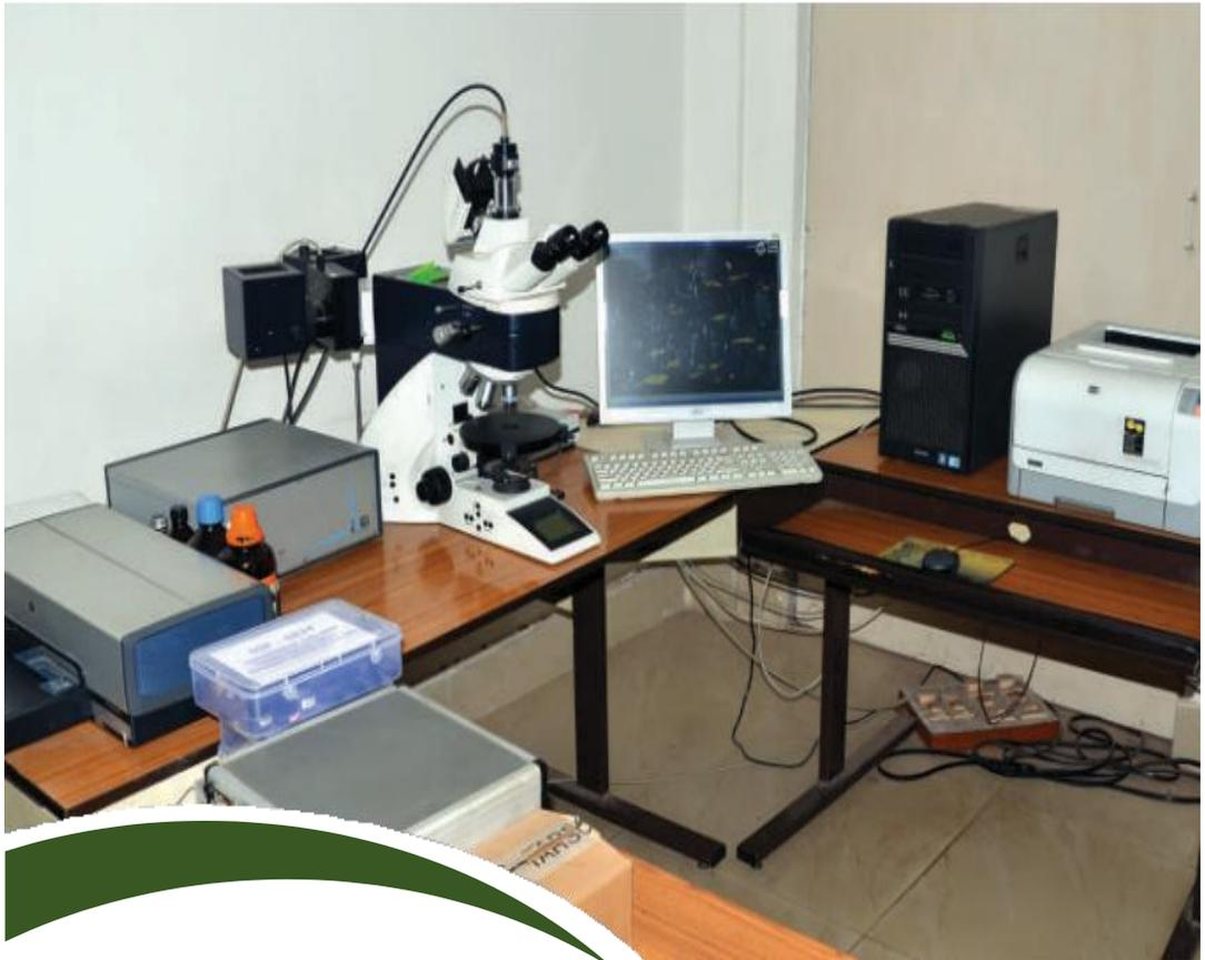
It is the most advanced version of Polarized Light Petrological Microscope, manufactured by M/s Leica, Germany. It has high-resolution optical devices operating under reflected as well as cross-polarized light modes. Through this, we can have images up to 500 magnification and measure the reflectance/rank of coal macerals as well as have modal counting of macerals and mineral matter on a visual basis.
