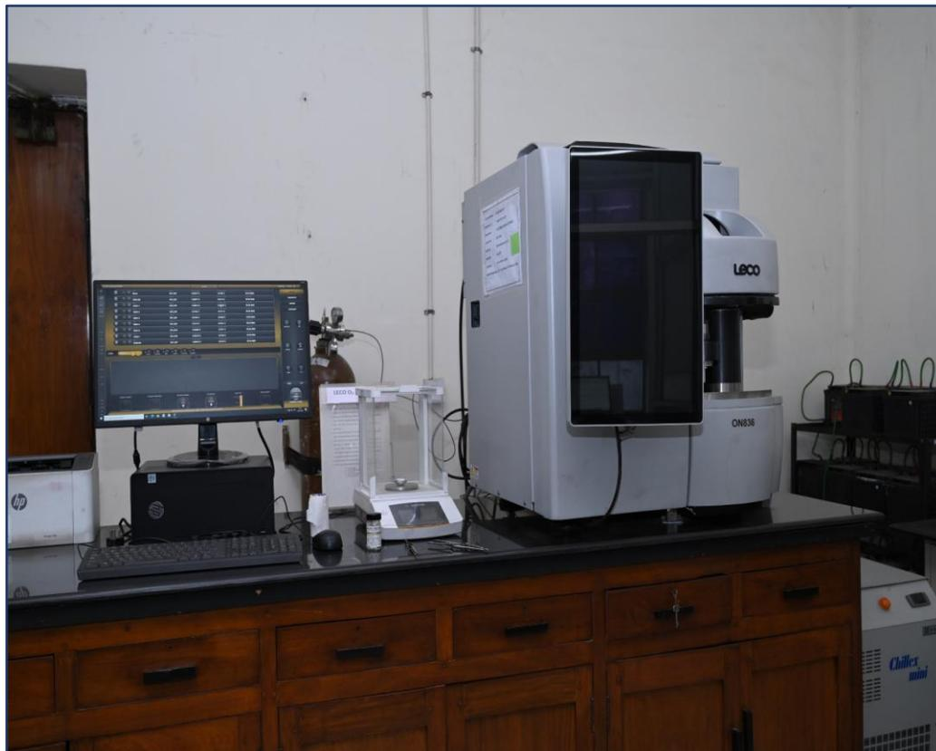
Elemental Analyzer is designed for wide-range measurement of oxygen, nitrogen content in steel and other metal, ferrous and nonferrous alloys using the inert gas fusion technique. This instrument has Automation and Cornerstone brand touch-screen software together to streamline the analysis, while a robust design ensures reliability.
