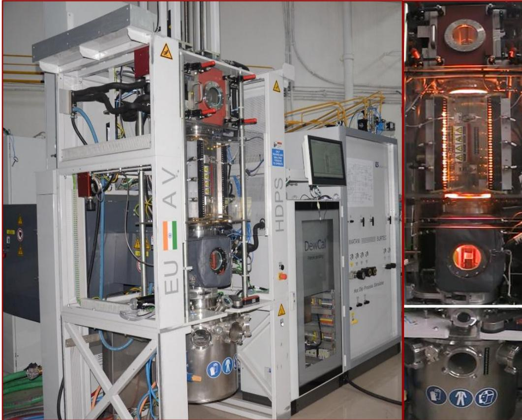
The state-of-the-art national facility, HDPS, can provide a comprehensive solution to industrial issues. It performs a realistic simulation of thermal treatment, galvanizing, galvannealing, and aluminizing processes for Advanced High Strength Steels (AHSS). The optimized process parameters can be directly transferred to the plant for trial.
