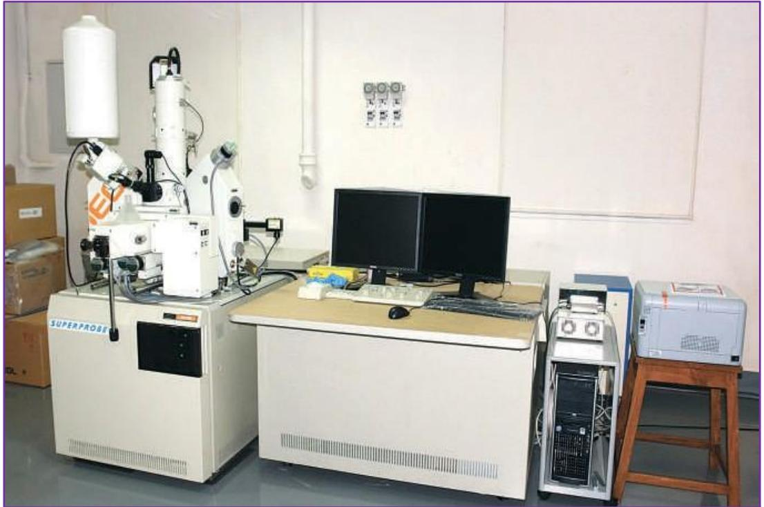
Electron Probe Micro Analyzer (EPMA) is a high-resolution elemental analysis instrument combined with wavelength dispersive X-ray spectrometers (WDS) and energy dispersive (EDS) analyzer. It can analyze elements both qualitatively and quantitatively. Depending on the requirement Wand La86 filament can be used. Point, line, and area analyses are possible, also, elemental distribution can be identified by map analysis. The minimum probe size is 0.5 microns (region of analysis).
