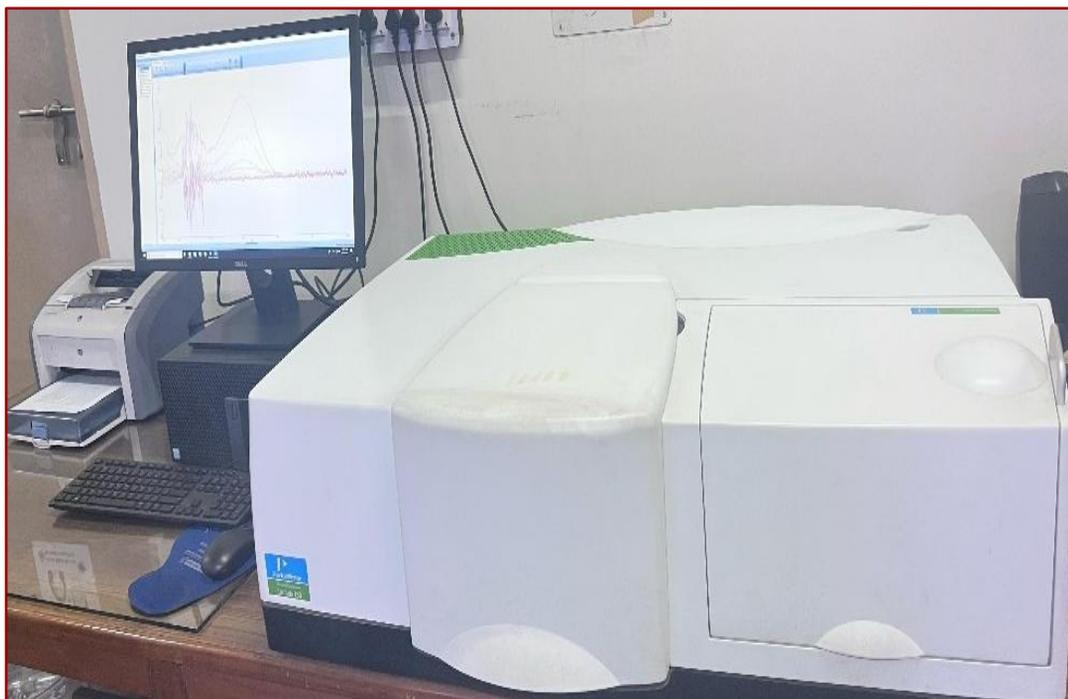
Double monochromator with solid-state facility. Present equipment, which is highly sensitive and low-noise, can give accurate results for even minimum concentration measurements. To calculate the band gap of semiconductors, oxidation state & concentration of transition metals.
