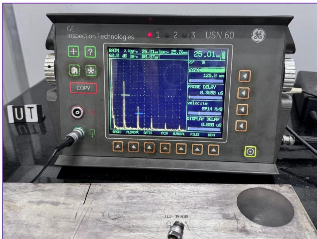
Ultrasonic flaw detector is used to evaluate materials in terms of defects, discontinuities, cracks etc. Various types of elastic modulus can also be determined by evaluating longitudinal and shear wave propagation velocities in materials. Frequency range of the system is up to 25 MHz with a maximum pulser voltage of 450 V. The system is equipped with an analog output port which can be used to save ASCII data for further analysis.
