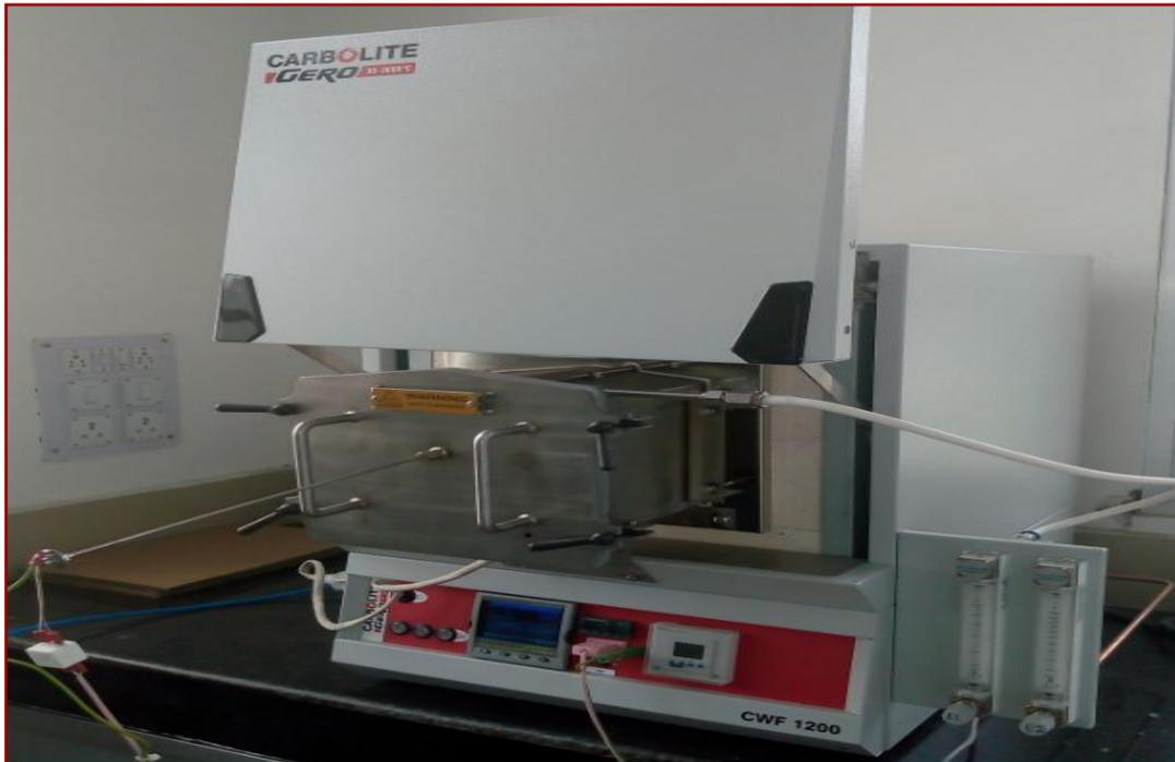
To perform high temperature corrosion studies on metals/alloys by means of creating a variety of reactive atmospheres such as (i) Oxidizing (ii) Flue gas within the convenience of an enclosed test facility with controlled flow rate.
