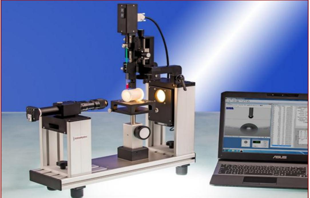
Sample table horizontally movable (magnetic slide system) and adjustable vertically with precision mechanics.
