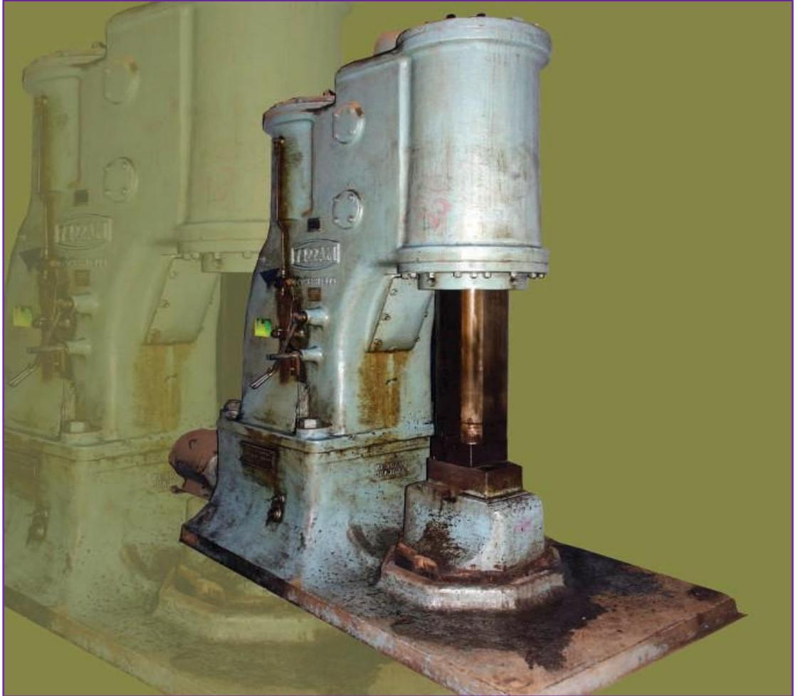
Three Pneumatic power hammers of 1 ton, 0.5 ton and 0.1 ton capacities have been used for open die forging.
