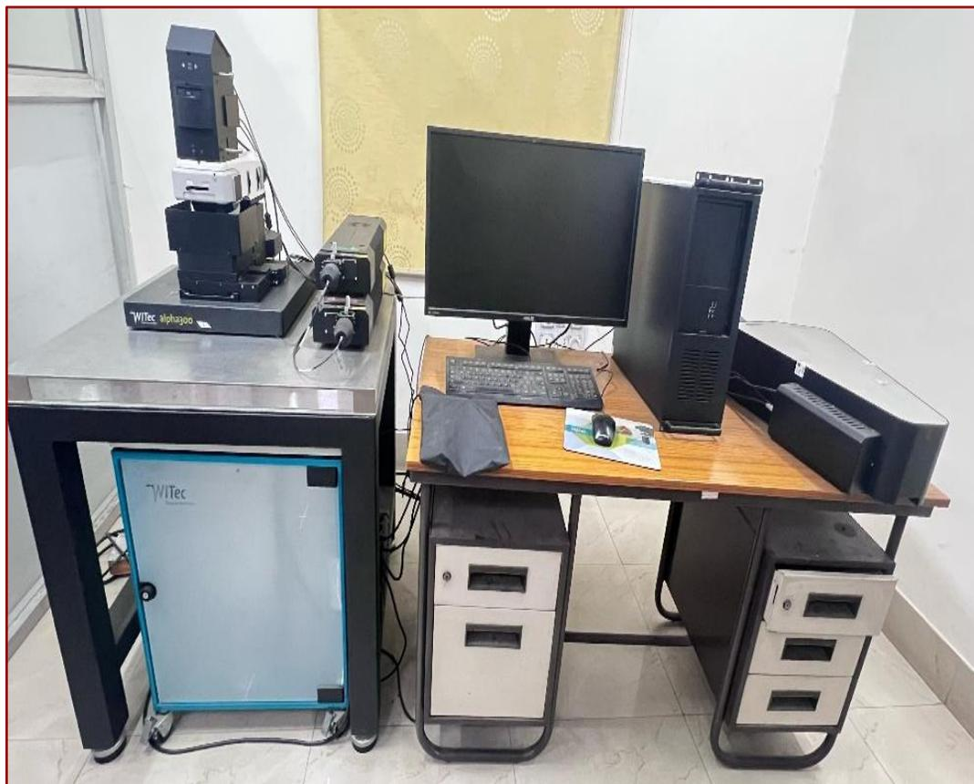
Equipment is equipped with 532 nm and 633 nm lasers. It can directly analyze the flat metallic surface, thin film, and powder samples without sample preparation. It can be used to monitor the in-situ corrosion product on the metallic surface after exposure to a certain environment. Raman spectra can be recorded at different locations by selecting the specific particles/ area through a confocal microscope, which can help to monitor different molecular structure formation and growth.
