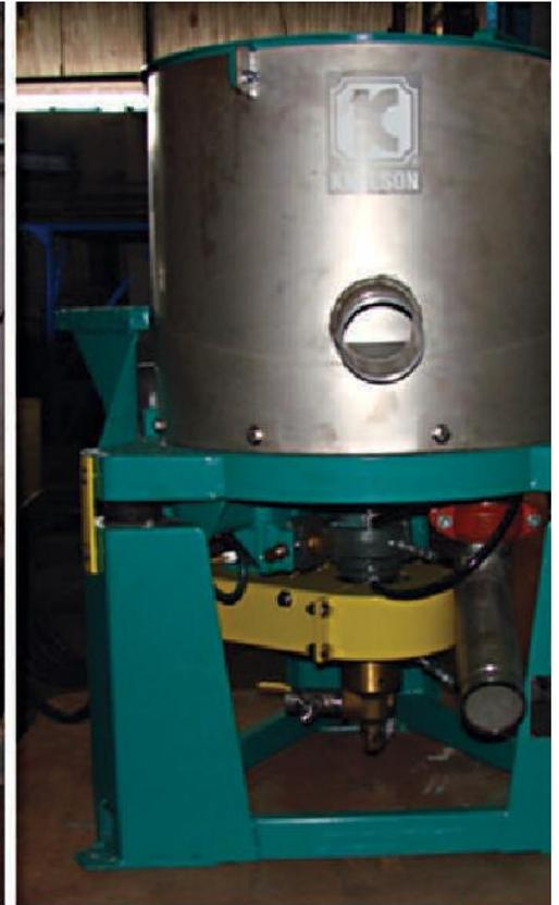
Knelson Gravity Concentrator is a Continuous Centrifugal Gravity Concentrator which utilizes the fluidization technology for high-mass yield recovery application. Knelson Concentrator is used primarily for bulk recovery of gold, PGE and various base metals and industrial minerals such as Copper, Chromite, Iron ore & Coal. It uses centrifugal force field to enhance the settling kinetics of fine particles to improve their recovery.
