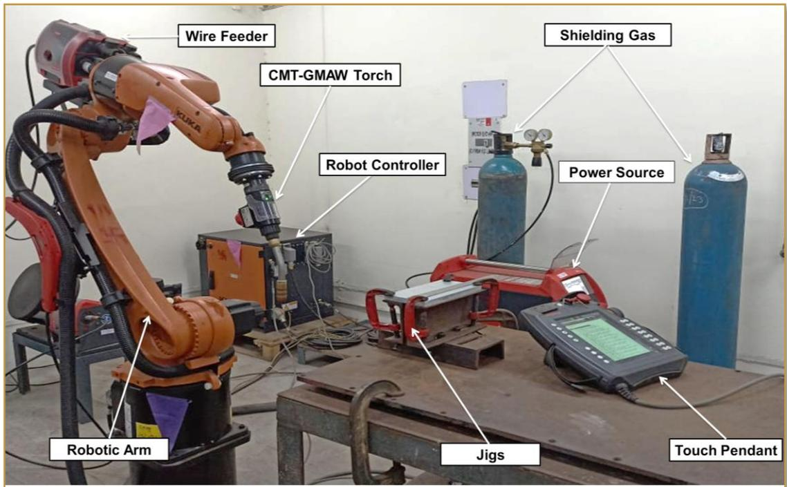
Wire Arc Additive Manufacturing (WAAM) is an advanced direct energy deposition (DED) process used to fabricate large-scale 3D metal or alloy parts with high productivity and cost-effectiveness.
