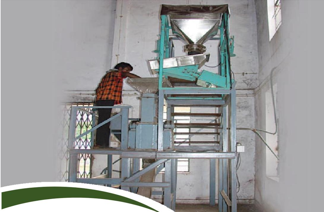
The impact hammer mill generates uniform product size with less fines due to shatter fracture. It can treat all types of ores at about 200 kg/h in continuous manner. The top size of the feed material is 100 mm. It can generate a product of less than 5 mm size. It has provision to introduce the feed through a vibratory feeder. The grate opening at the discharge can also be changed to restrict the top size of the product. The rotor speed can also be controlled from the control panel.
