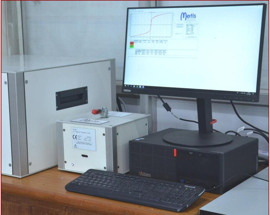
Measurement Platform for the determination of AC magnetic characteristics of soft magnetic materials like soft ribbons & foils.
