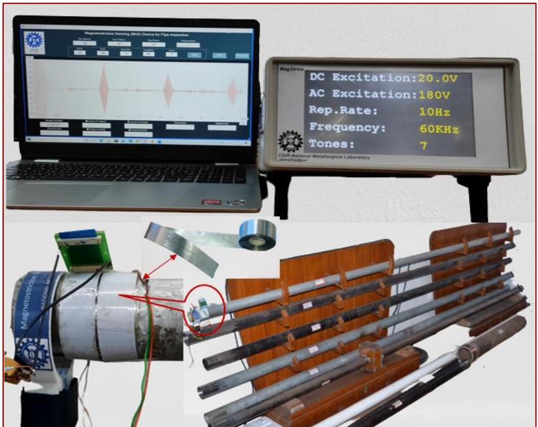
The electromagnetic sensing device generates mechanical waves in pipes and also picks up reflected signals using amorphous soft magnetic ribbons as sensor elements.
