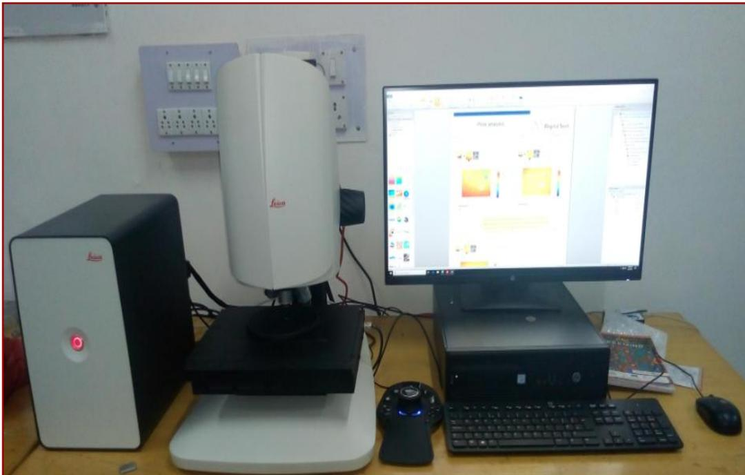
Combines confocal metrology in HD with interferometry to a versatile dual-core system. High-performance software, simple module selection with one click, and confocal scanning without movable parts with vertical resolution up to 2nm for surfaces with sloping areas and intricate structures. Interferometry with a resolution up to 0.1 mm for even surfaces with microstructures.
