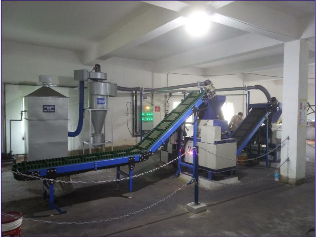
This is a battery dismantling cum processing facility which is capable of processing spent batteries to the tune of 1 ton/day and generates black mass (<math>< 50 \mu\text{m}</math>) devoid of copper, aluminium and iron contamination. This facility is available under HOT mode for recyclers and entrepreneurs.
