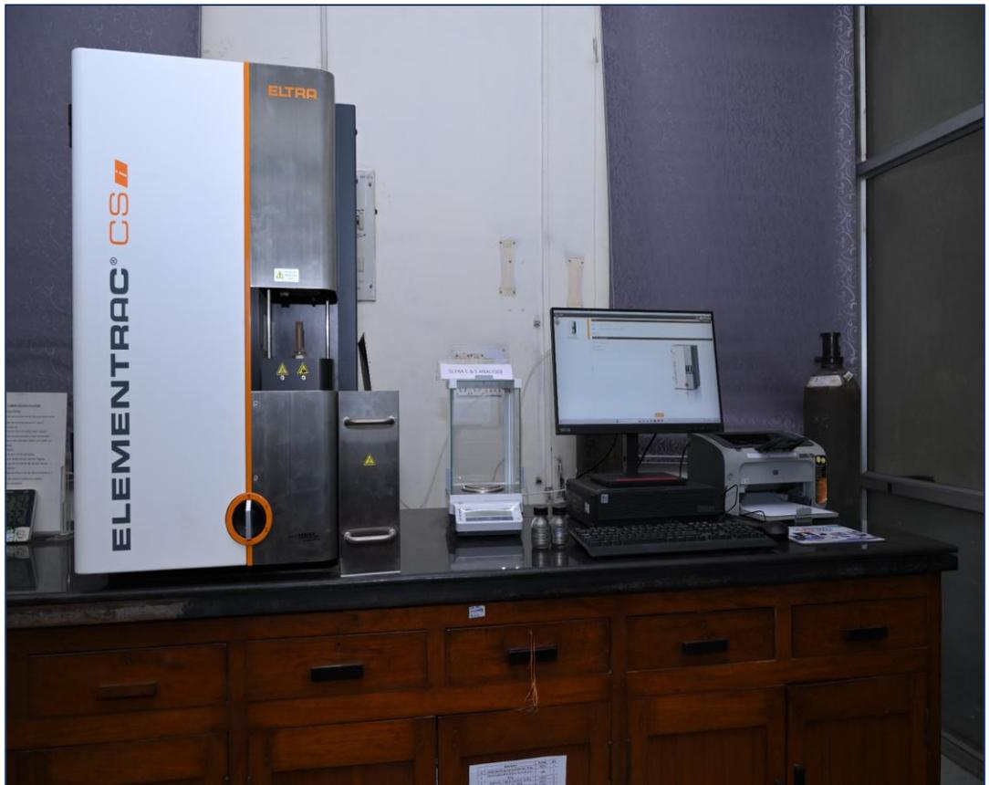
The elemental analyzer ELEMENTRAC CS-i measures the Carbon and Sulfur concentration in predominantly inorganic samples through combustion in an induction furnace and the subsequent analysis of the gaseous combustion products carbon dioxide and sulfur dioxide. The high temperature of more than 2000°C ensures complete decomposition of the sample and thus reliable and accurate elemental analysis over a wide concentration range.
