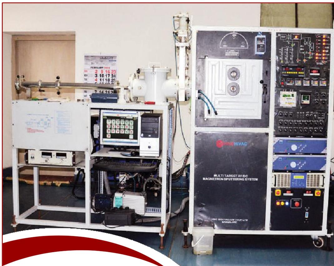
The magnetron sputtering can be used for coating single layer and multilayers of metals, alloys, ceramics, and some high-temperature polymers such as Teflon, etc. It is an atomic deposition PVD process, done by plasma generation. The unit has the capability of  $1 \times 10^{-6}$  mbar. It has 3 magnetron sources with a substrate holder having substrate heating and biasing facilities up to  $700^{\circ}\text{C}$  and 200 V, respectively.
