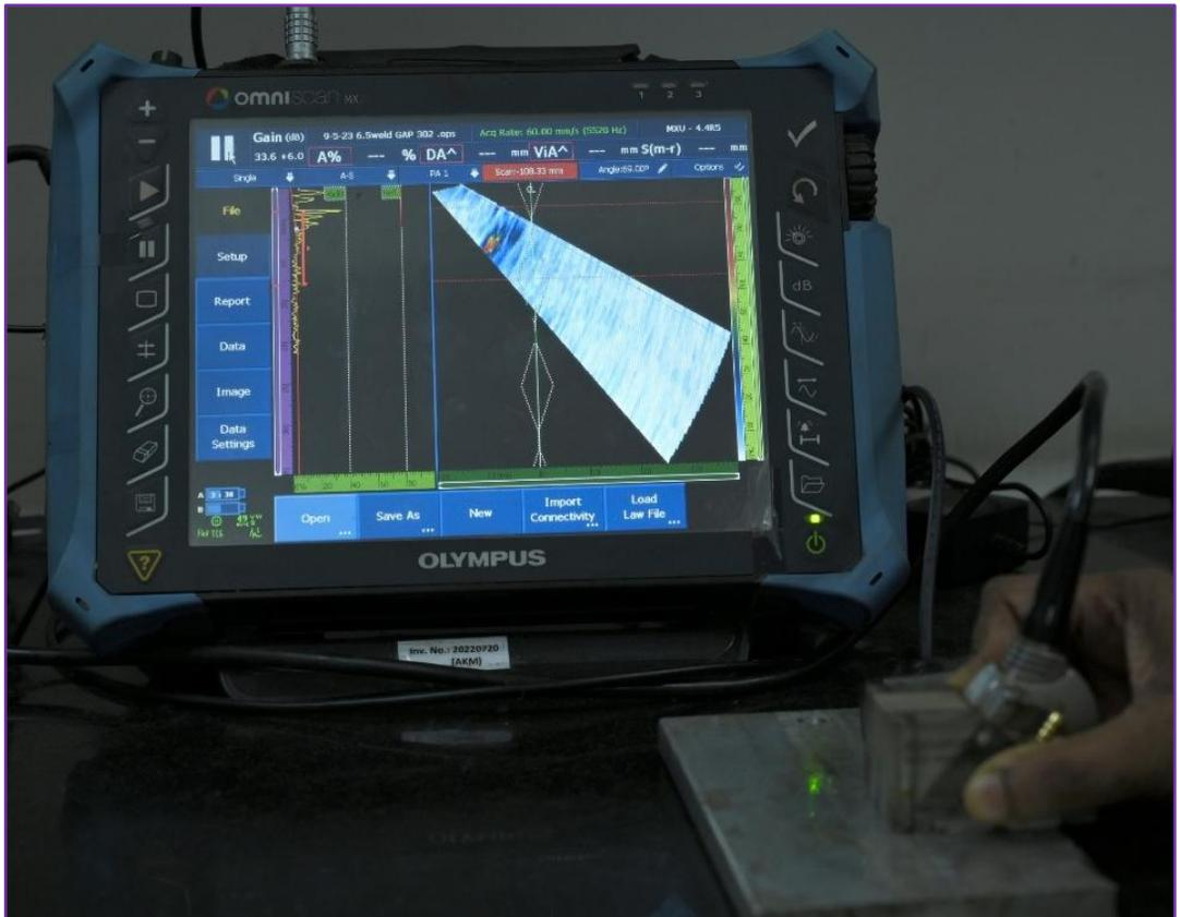
Phased Array Ultrasonic system is an advanced nondestructive testing method which uses array of transducers to steer and focus beams electronically, enabling detailed inspection of materials and structures without causing damage. Ultrasonic beams can be steered, scanned, swept and focused without moving the transducers that makes this technique superior to conventional angle beam ultrasonic technique.
