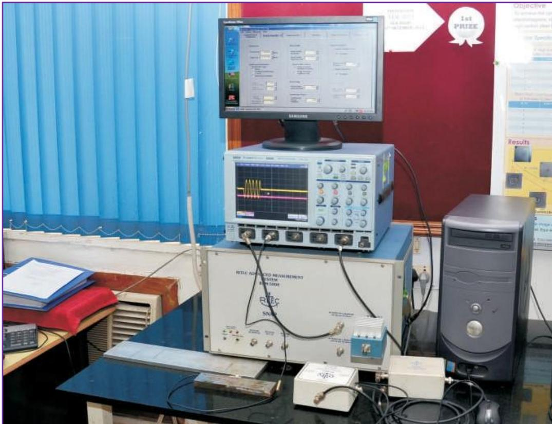
It is a high-power RF tone burst generator with an output of 5 kW up to 7 MHz. The system operates at a Frequency Range of 40 kHz - 20 MHz. It can be used to characterize material by measuring non-linear properties. It examines harmonic frequencies for increased sensitivity in material evaluation
