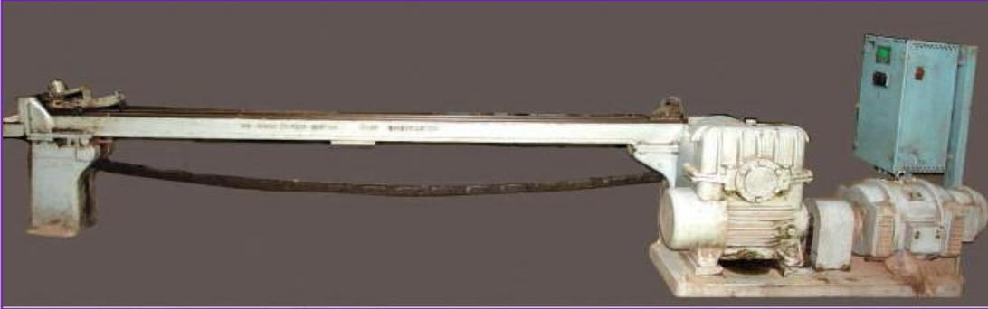
Bench-type wire drawing machines is used for drawing ferrous as well as nonferrous materials. In the present setup, wires up to 0.3 mm in diameter can be drawn.
