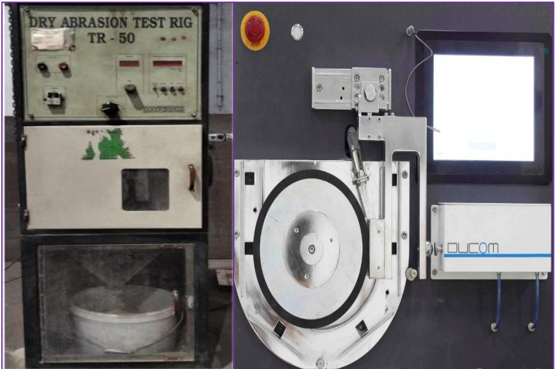
The Dry Abrasion Testing (TR50) Machine is a precision instrument designed to evaluate the wear resistance of materials under dry abrasive conditions. It operates by subjecting test samples to controlled abrasive forces, simulating real-world wear scenarios.
