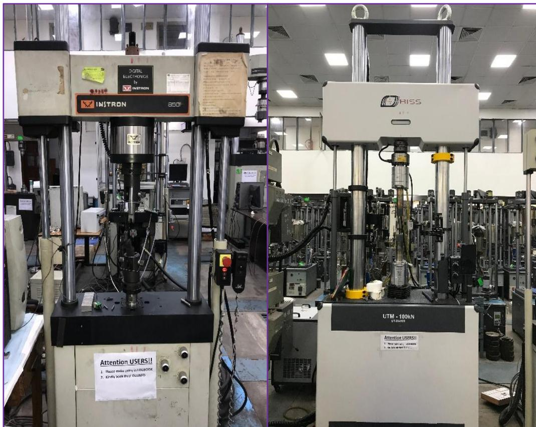
CSIR-NML has 3 numbers of dedicated Creep-Fatigue Test systems of 3.2 T and 10 T capacity with furnace (1100°C) and side entry type high temperature extensometer. The function generator of the system can produce different types of waveforms with long hold time (100 hrs) at either or both peaks.
