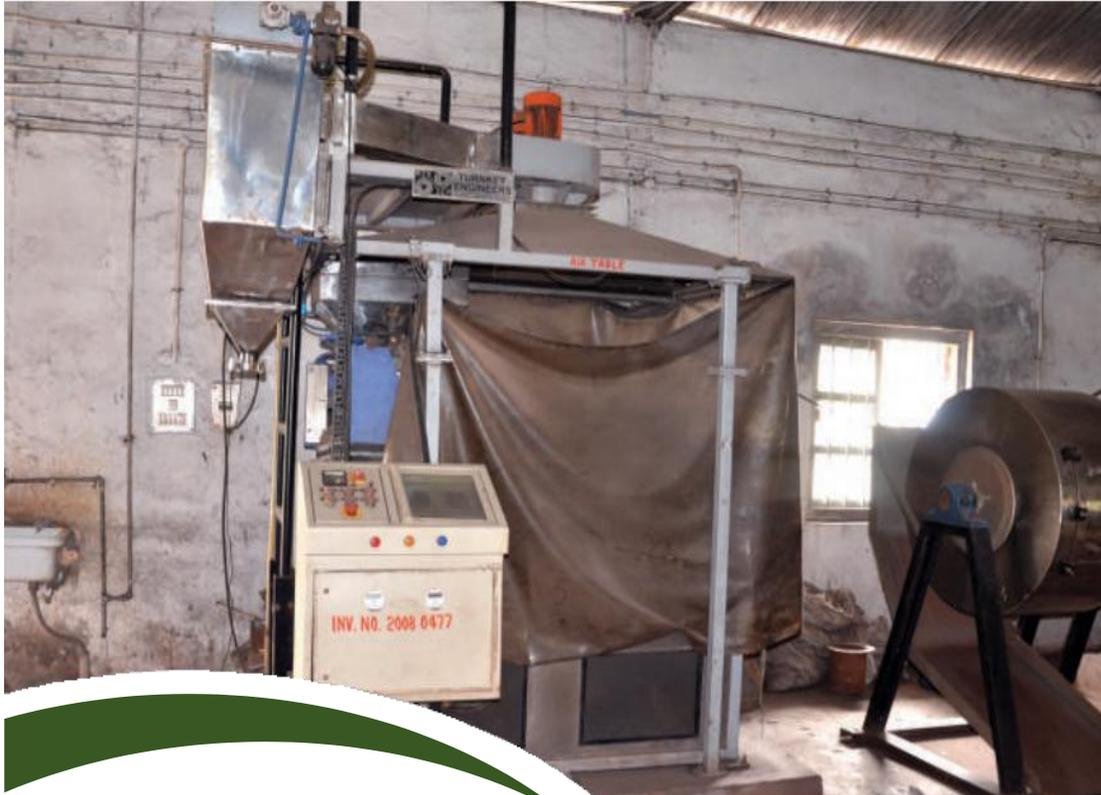
Fluidized Bed Separator/ Air Table is primarily utilized for separation of dry uniformly sized solid particles with differential specific gravity. Air-pulsed fluidization is triggered by air stream and guided into the separating deck. The principle of separation is defined as follows:
