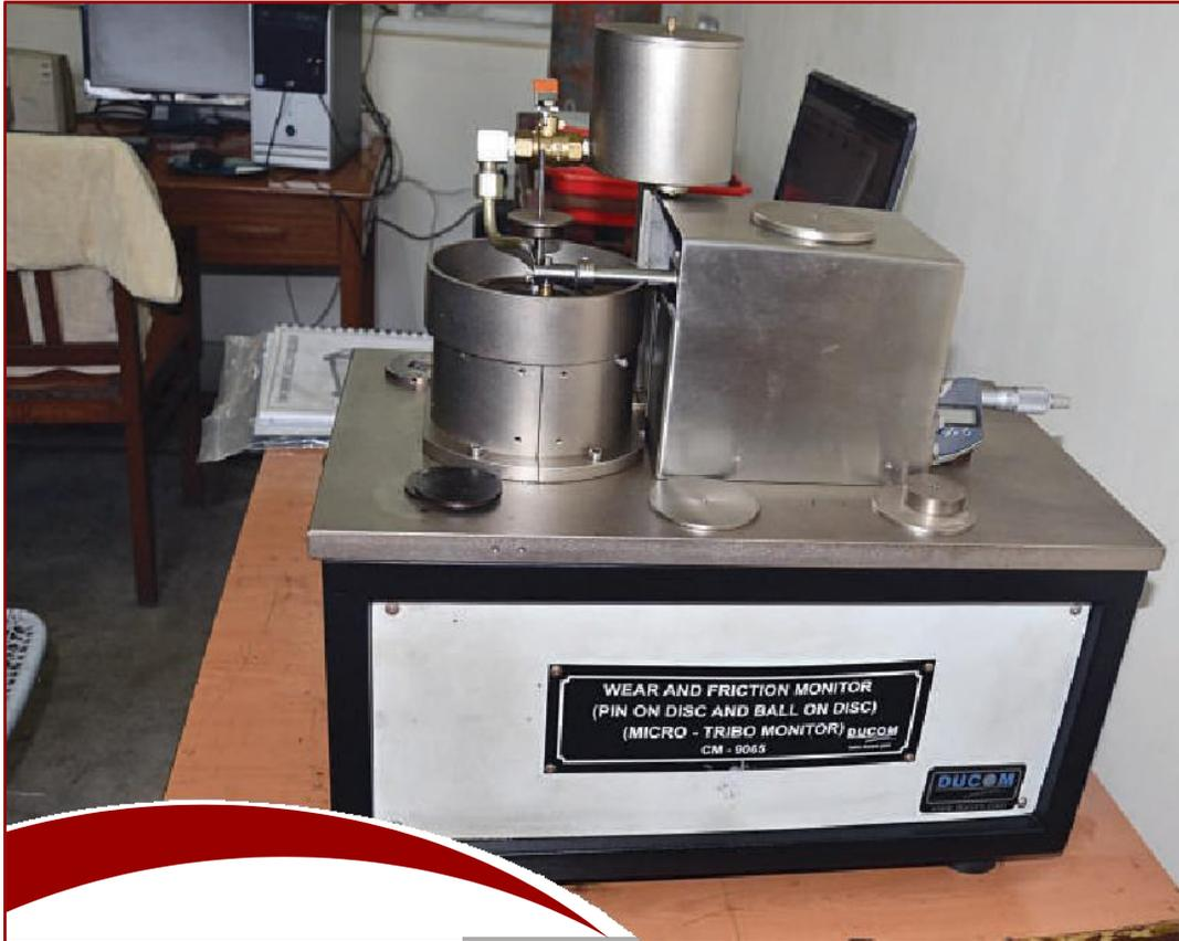
Pin-on-Disc wear tester is used to study the material loss due to frictional forces between the two moving bodies in contact. The system is capable of measuring simultaneously the friction coefficient and wear loss with time or sliding distance under varying load. The lubricability of the fluid can also be evaluated.
