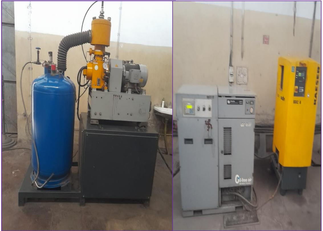
A liquid nitrogen plant produces liquid nitrogen at a temperature of  $-40^{\circ}\text{C}$ . This liquid nitrogen is used for sub-zero temperature testing and sophisticated equipment cooling, etc.
