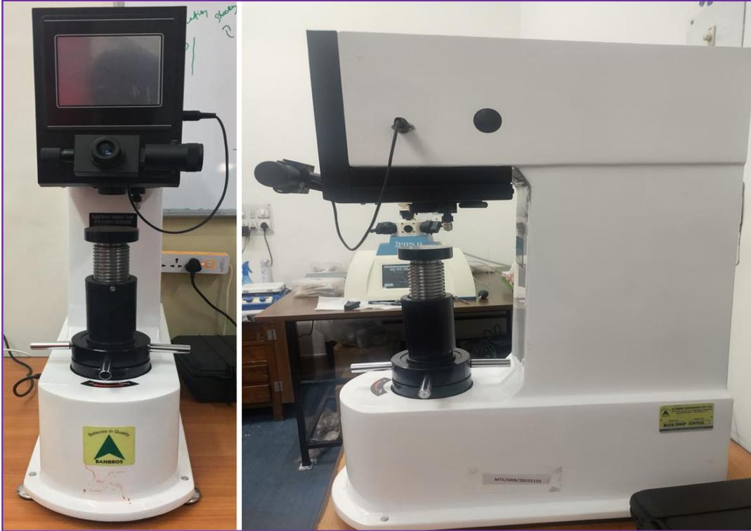
This equipment is capable of automatically measuring the hardness of various solid materials with hardness up to 600 HBW. Users can select from different combinations of tungsten carbide indenter ball diameters (2.5 mm, 5 mm, and 10 mm) and test forces/loads (ranging from 62.5 to 3000 kgf) based on their specific requirements.
