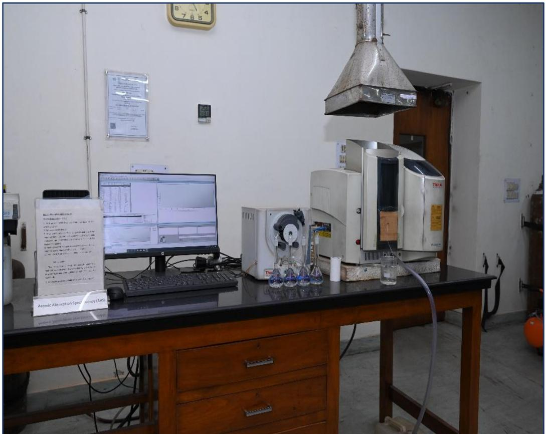
Atomic Absorption Spectroscopy (AAS) detects elements in either liquid or solid samples through the application of characteristics wavelength of electromagnetic radiation from the light source. Individual elements will absorb wavelengths differently and this absorbance are measured against standards.
