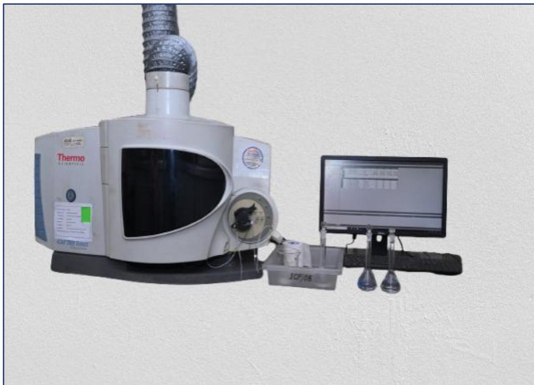
The iCAP7600 series of ICP OES is a powerful dual-view spectrometer, which is used for the analysis of trace, minor & major elements present in aqueous samples like Water, wastewater, leachate, etc. Analysis of Mineral, Ores, Metals, Steel, and other Alloy samples can also be done after their digestion in suitable acid reagents.
