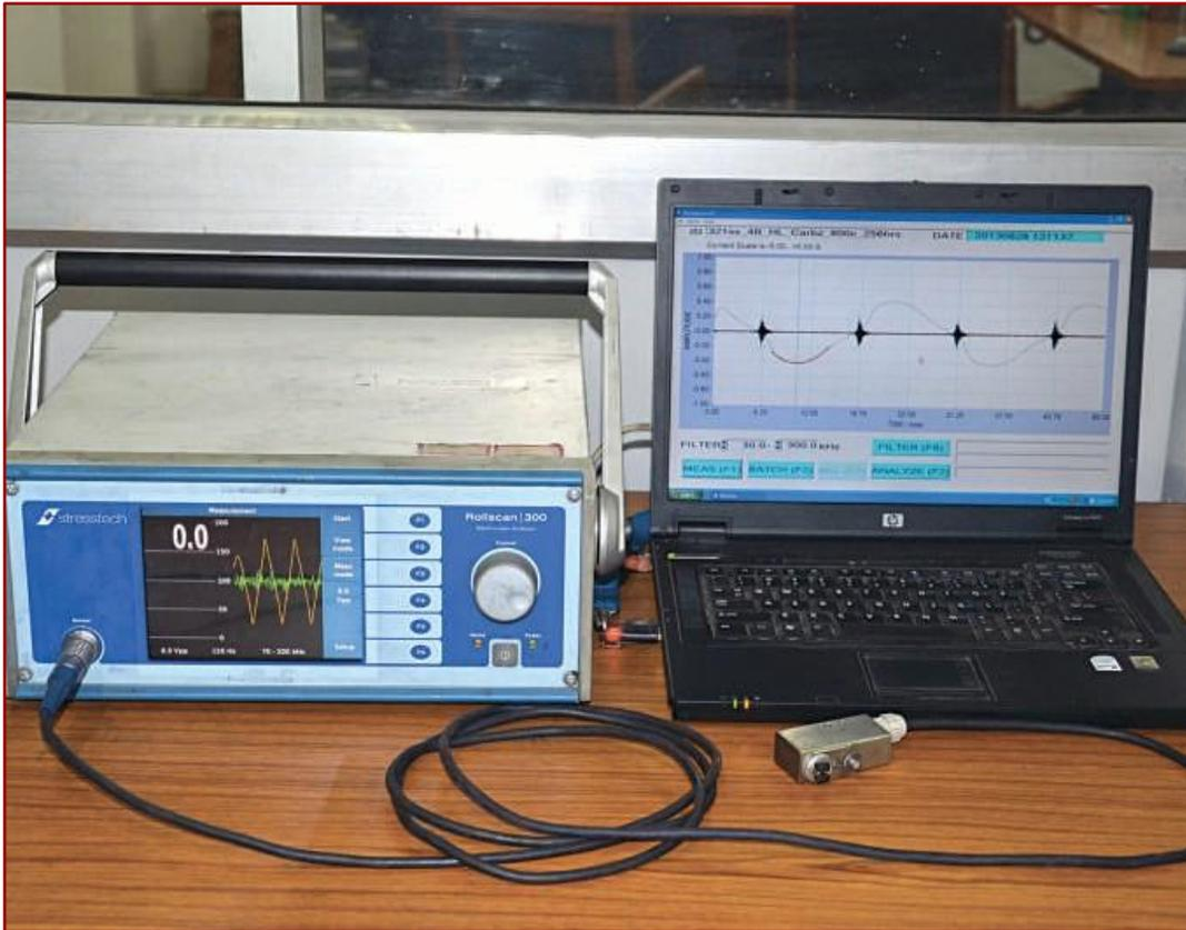
The Magnetic Barkhausen emission (MBE) is measured by the instrument Rollscan 300, which is a digital Barkhausen noise analyzer. This instrument can be used for the measurement of the Magnetic Barkhausen Emission (MBE) signal. The effect of residual stress, creep, and fatigue on MBE signals of ferromagnetic materials can be studied.
