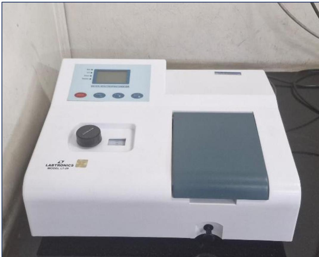
UV-Vis spectroscopy is an analytical technique that measures the amount of discrete wavelengths of UV or visible light that are absorbed by or transmitted through a sample in comparison to a reference or blank sample. This property is influenced by the sample composition, potentially providing information on what is in the sample and at what concentration. The instrument works on the principle of Beer-Lambert law.
