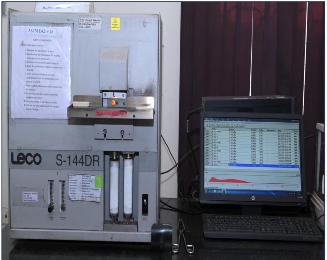
Sulfur analyzer is used to determine total sulfur content in coal. Coal is burnt in presence of excess oxygen and the SO<sub>2</sub> gas produced is analyzed using IR detector. The analysis is fast with each sample taking 3 min approximately.
