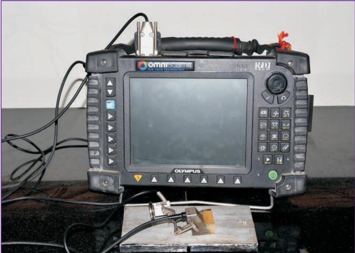
Ultrasonic system with Time-of-flight diffraction (TOFD) is a technique that uses two probes in pitch-catch mode and detects and records signals diffracted from defect tips allowing both detection and sizing. The TOFD data is displayed in a gray scale B-scan view. TOFD offers wide coverage and amplitude-independent sizing complying with the ASME 2235 code.
